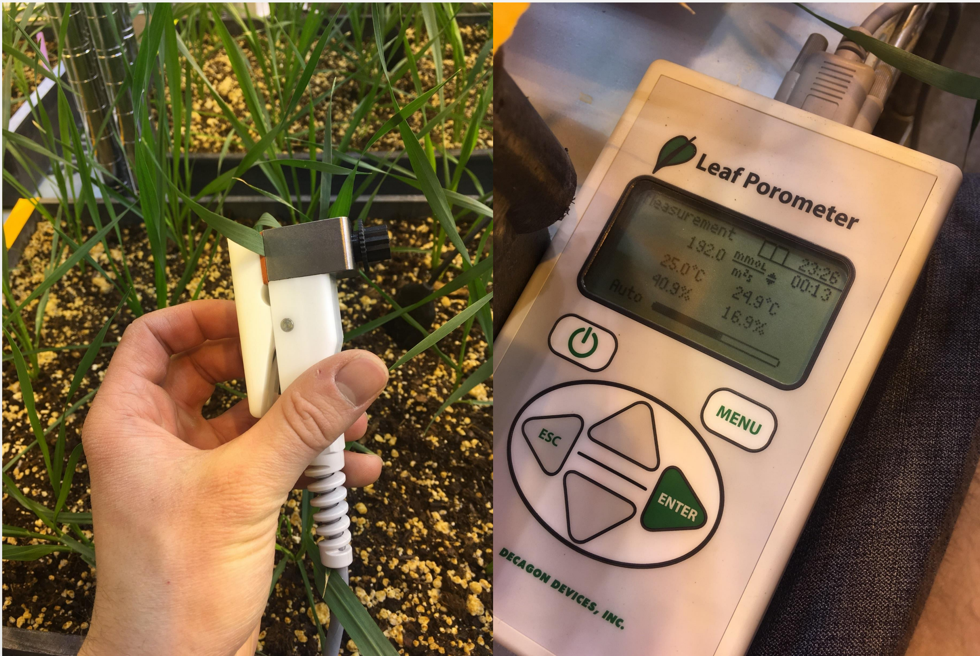
Taking stomatal conductance of wheat plants in experiment (left) with the leaf porometer machine (right)
