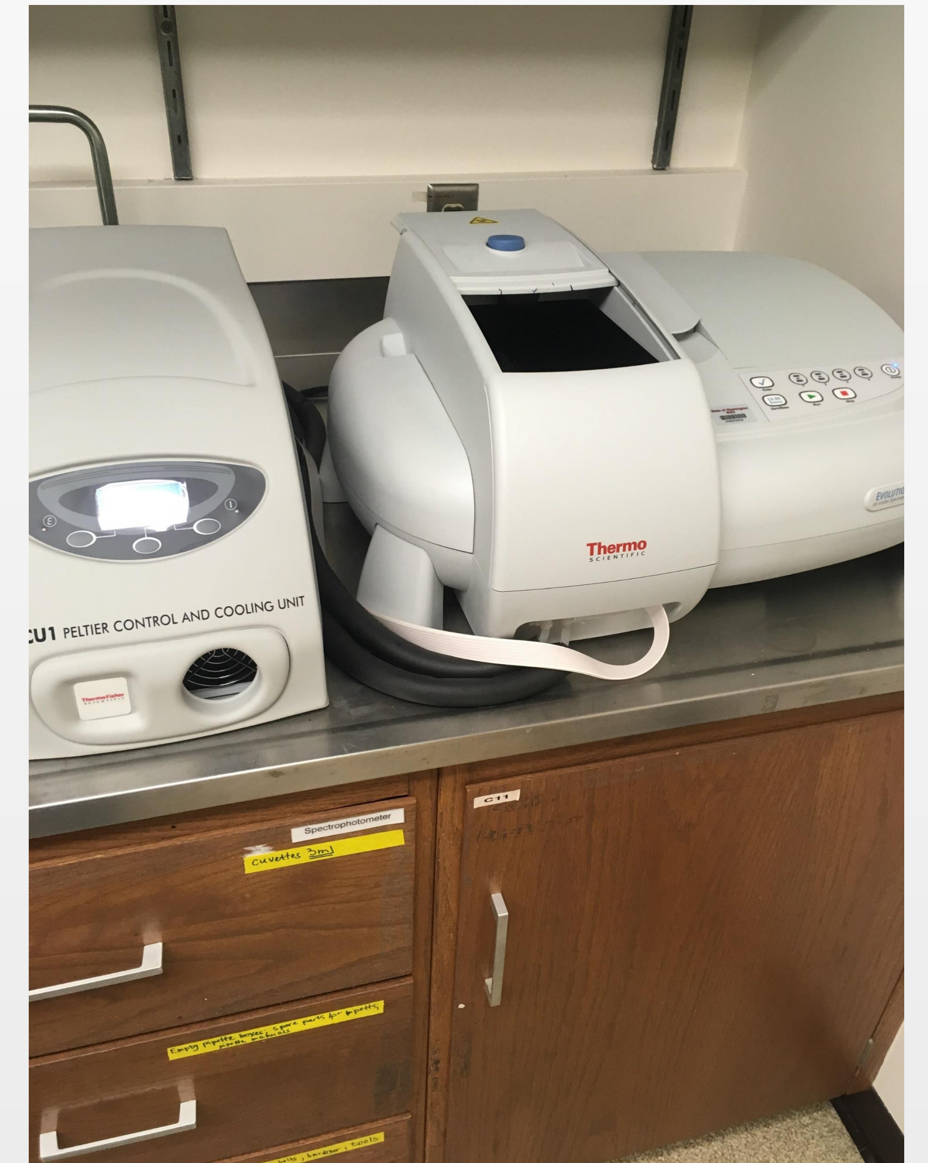
Spectrofluorometer, the piece of equipment that measures absorbance of various assays I ran
