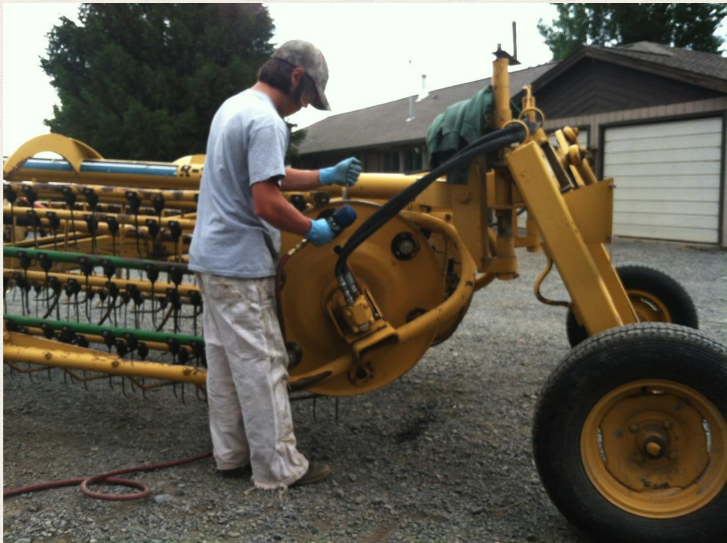
During the first cutting of the season, our rotary hay rake broke down. This yellow rake was purchased to replace the broken rake. In this picture I am replacing failed bearings with updated units.
