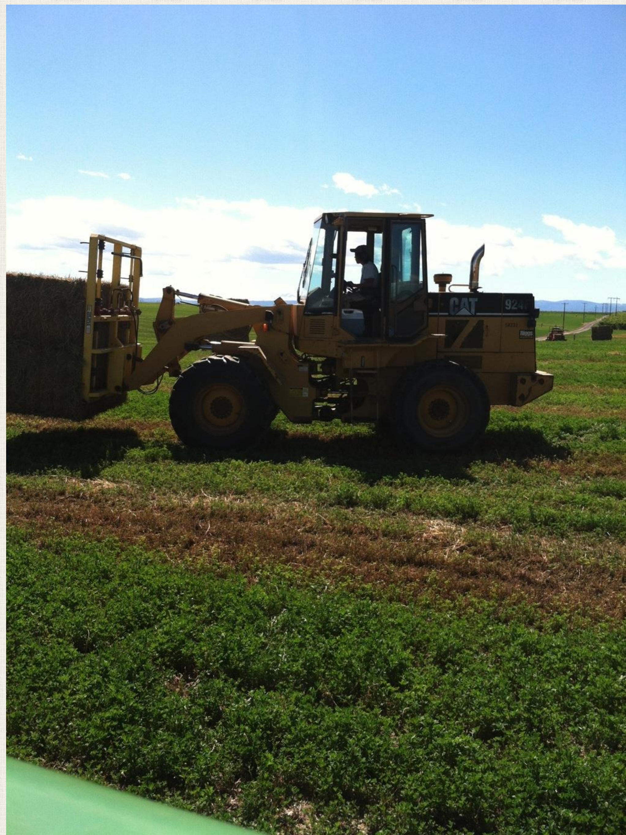
During hay harvest, I ran the Cat 924F front loader with a hay head to stack and load the hay onto trucks.
