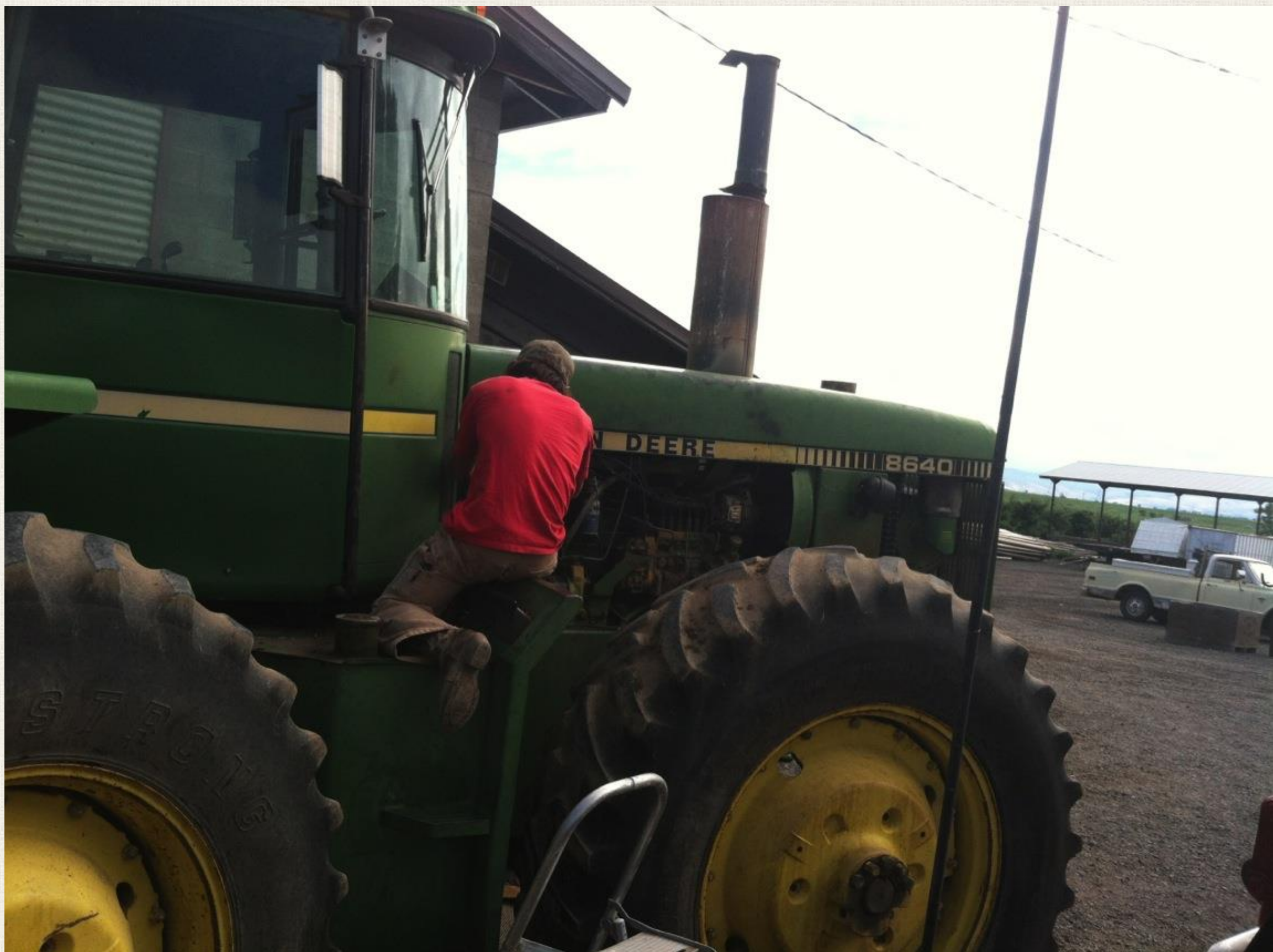
Removing the hood from this John Deere 8640. During the first cutting the PTO clutch failed and stuck on. While replacing the PTO clutch, we also repainted the hood, grilles, and side panels. We also replaced the leaky hydraulic pump, blew out the clogged radiator, and addressed a few other problems.
