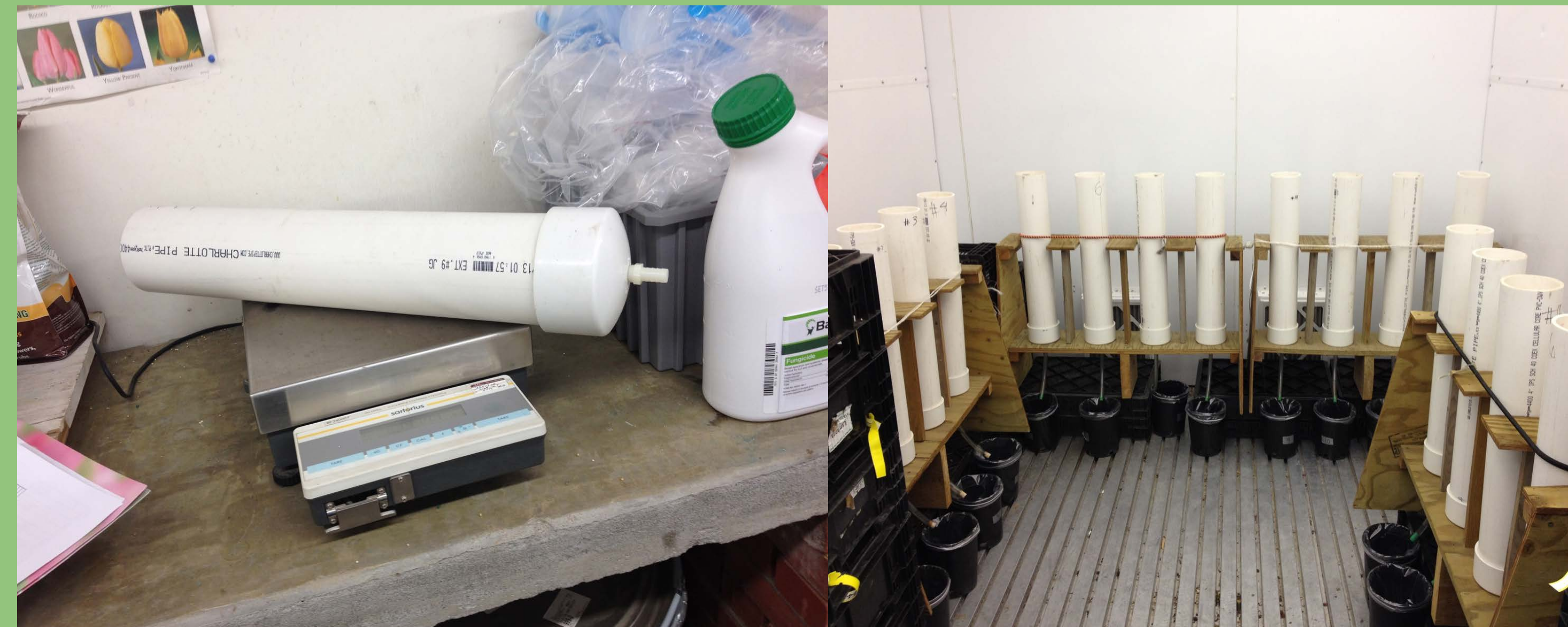
a. Set up the soil columns for the experiment
