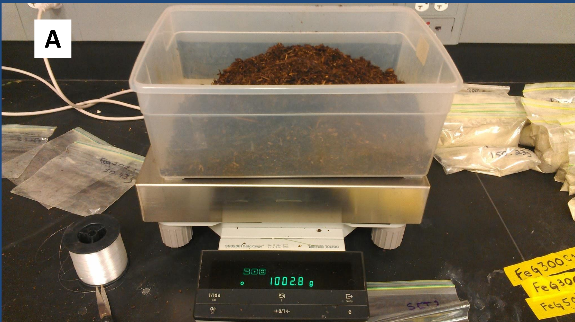
One of the projects I was involved with was making the compost batches with various iron sulfate and iron gluconate concentrations which are the ones used for evaluation of contaminated soil remediation. We used feedstock from the WSU composting facility as starting material. We weighed out about 1000 grams of feedstock, added the iron, and mixed thoroughly (A). Then placed the mixture in a bag with labels and tied them up (B). We then went to the WSU compost facility and buried them into the center of the pile where it is the hottest (C and (D)).
