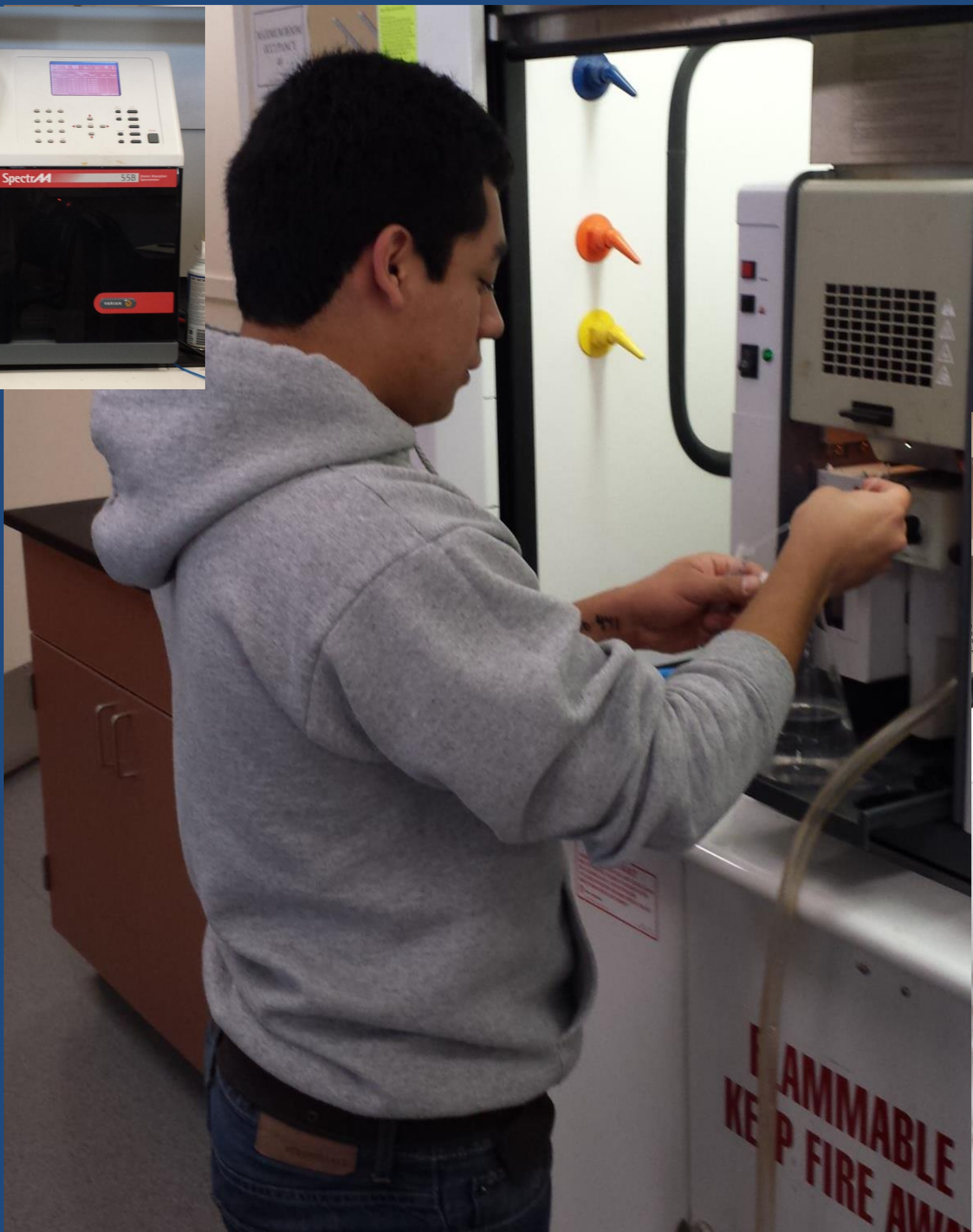
(Far Left) During my research experience I was able to learn and use an atomic absorption spectrometer, which is the machine we used to measure calcium, magnesium, and lead concentrations (middle). I was also able to use a Spectramax UV-Vis spectrometer to analyze phosphorous concentrations.
