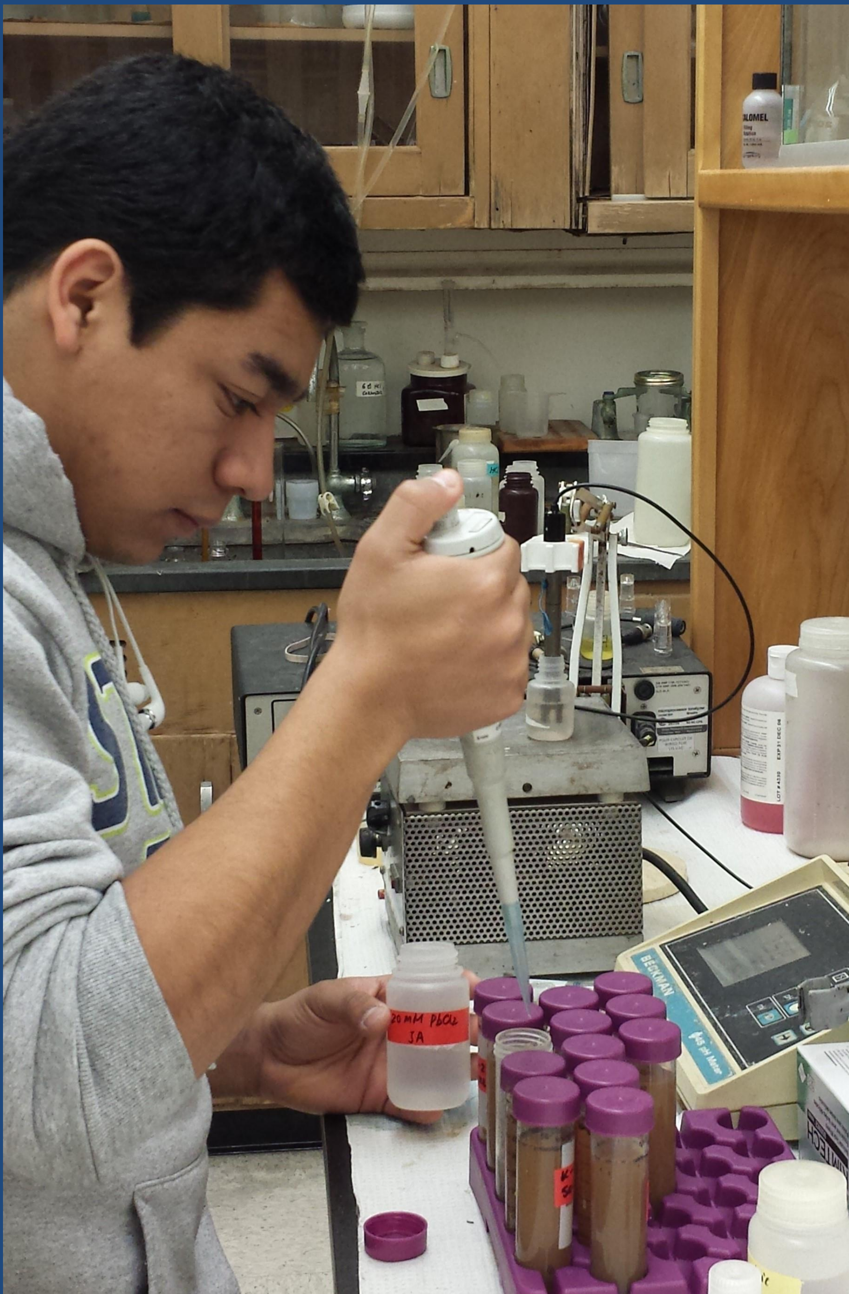
(Left) I am adding nitric acid to each of the samples to adjust the pH. For my project I had to pipette different chemicals into the samples depending on the experiment we were going to conduct. Sodium hydroxide or nitric acid was added to adjust the samples pHs. (Above) Samples are being filtered to collect the solutions and prevent soil particles from penetrating. The solutions were then analyzed for phosphorous, calcium, magnesium, carbon, and lead concentrations.
