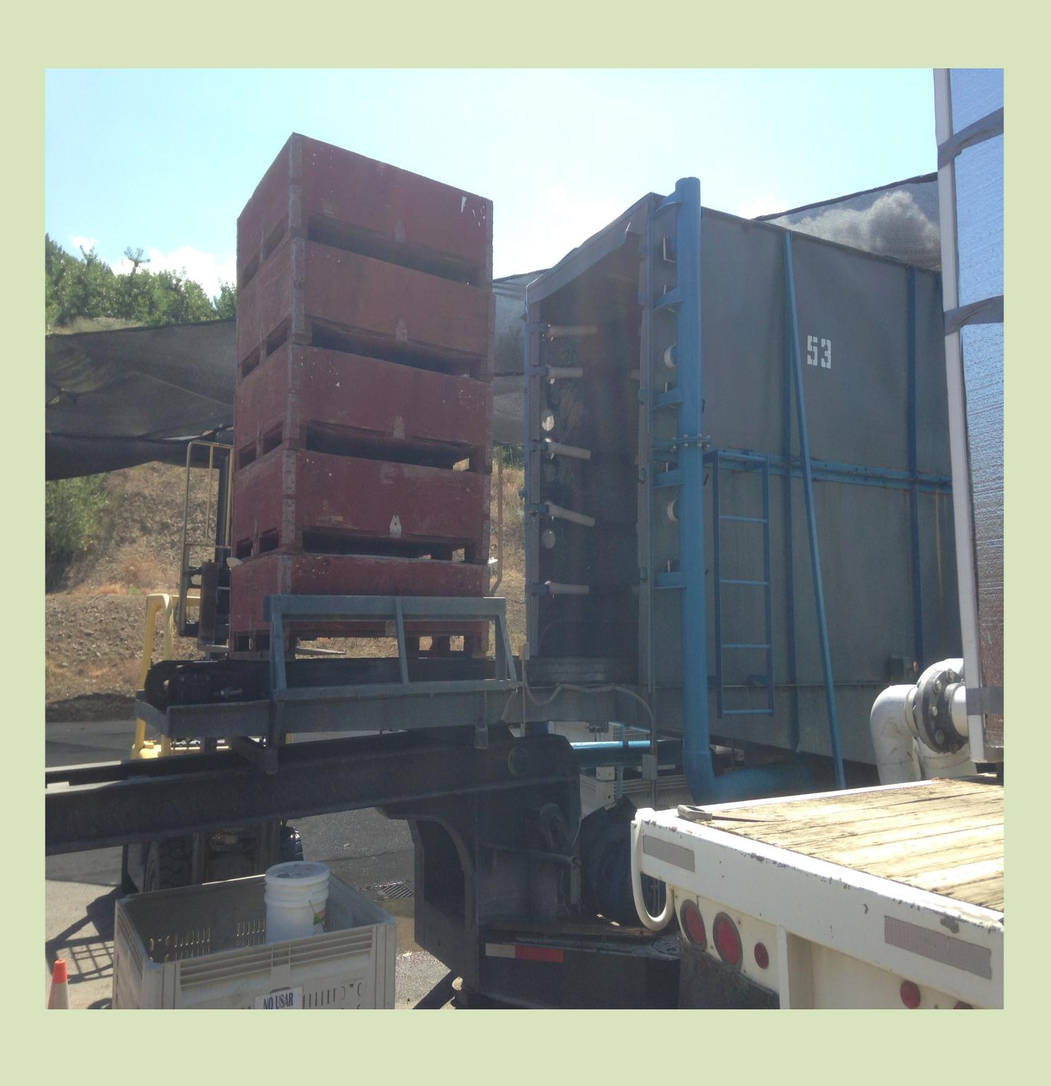
Here is a picture of cherries going through a Hydro Cooler. The cherries would drop in temperature 40 degrees after the fruit was put through this hydro cooler. The fruit would then be loaded on Semi- trucks and sent to the warehouse where it would be packed.
