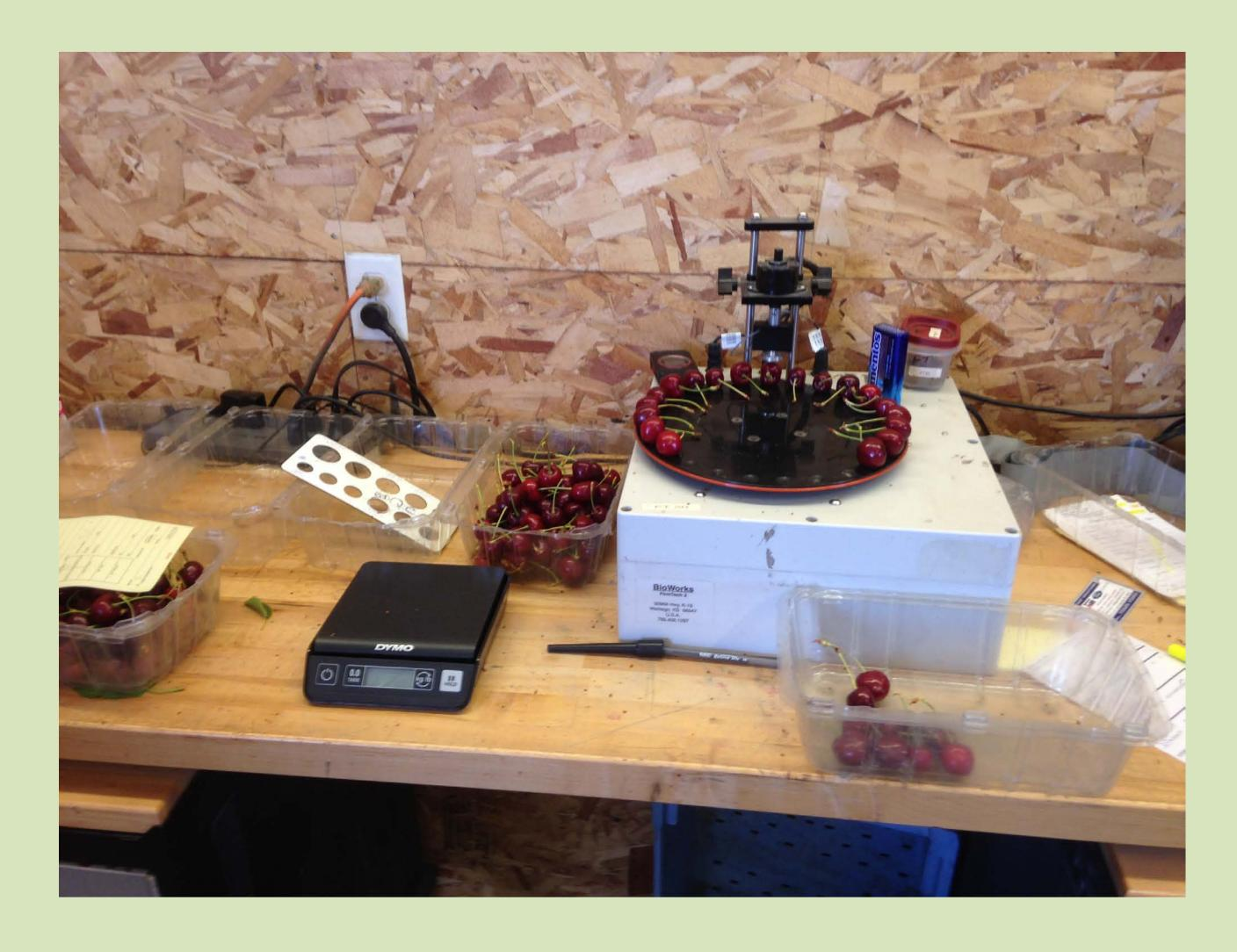
Here is a typical station for doing a fruit quality sample. The cherries would sorted in the plastic trays and then the clean cherries would be ran on the firmtech which would measure the size and the firmness of the cherry.
