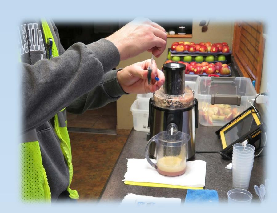
The picture on the **right** shows a refractometer. This is a common tool in the industry to test sugar content in fruit by pipetting a small amount of juice onto the testing area and pressing start. The units expressed are in percent brix which is simply grams of sucrose/100 grams of solution
