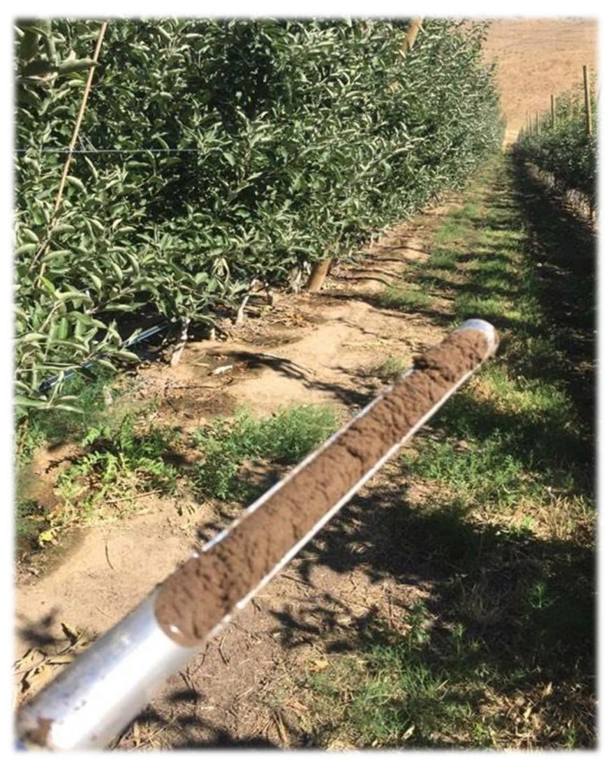
A soil sample collected with a soil probe.
