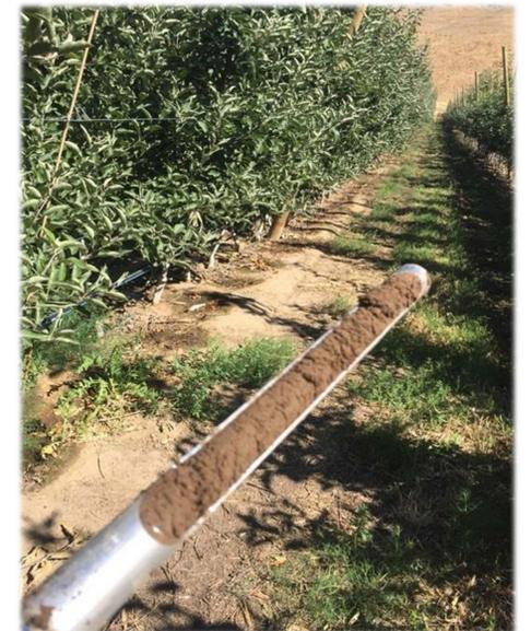
A soil sample collected with a soil probe.
